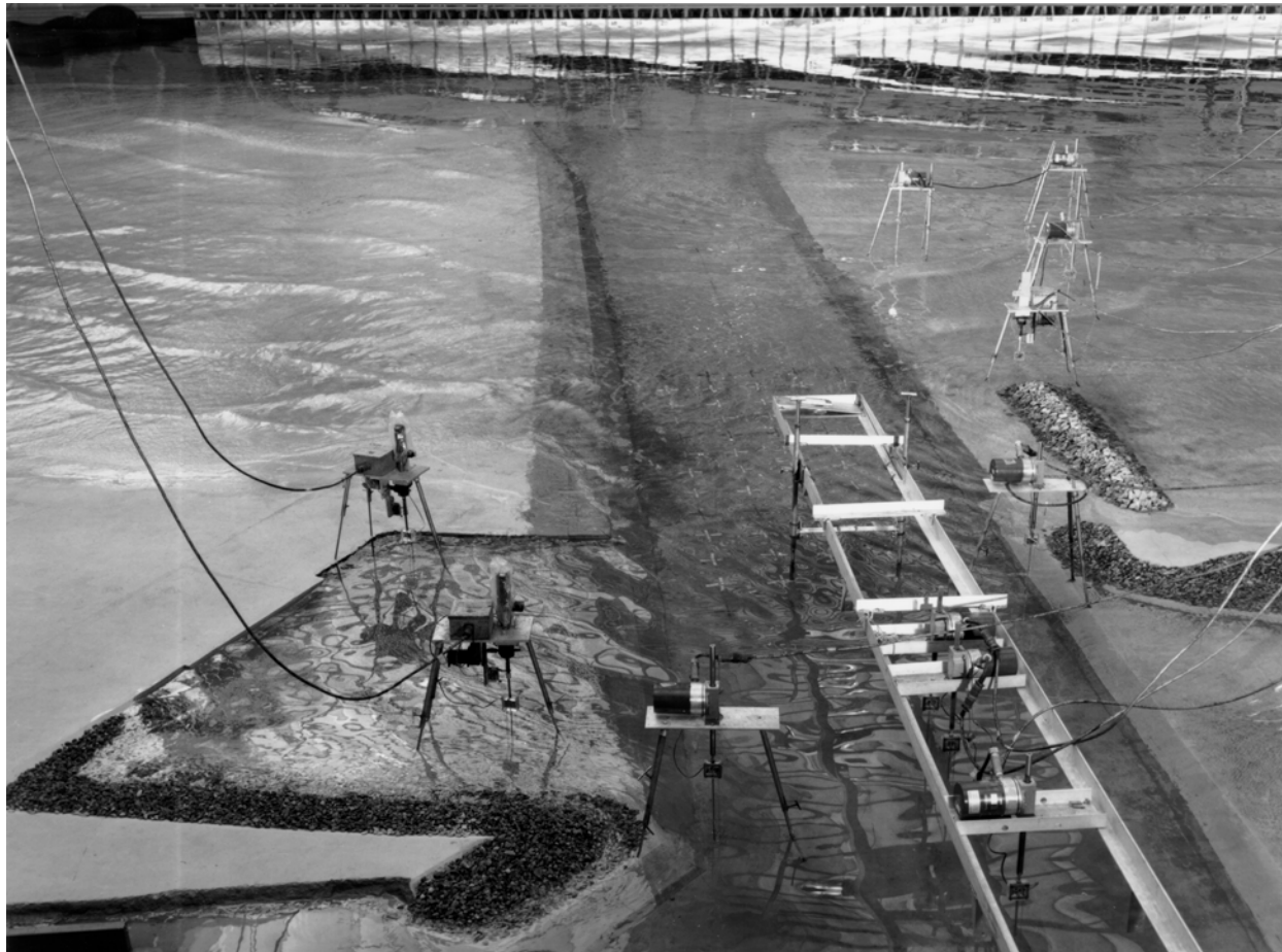
Figure II-7-35. Photograph of physical model, Barbers Point Harbor, HI (Briggs et al. 1994)
