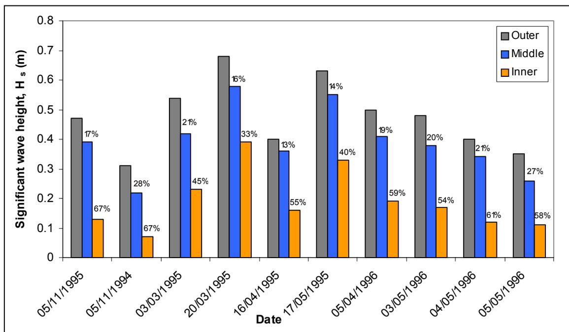
**Figure 2.4** Reduction of significant wave height between sandflat (outer), the saltmarsh edge (middle) and saltmarsh (inner) stations (from Möller *et al.* (1999))
