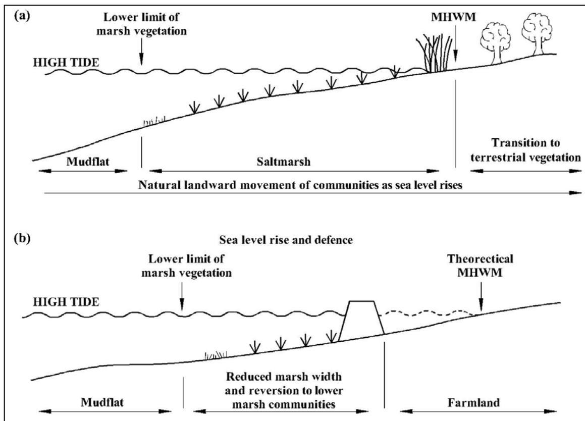
**Figure 4.2 Illustration of the concept of Coastal Squeeze (a) before construction of Sea Wall and (b) after construction (from French, 1997)**
