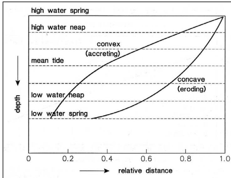
**Figure 2.2** Schematic diagram showing morphology of concave and convex mudflats relative to tide levels and relative shore-normal distance (after Van Rijn, 1998)
