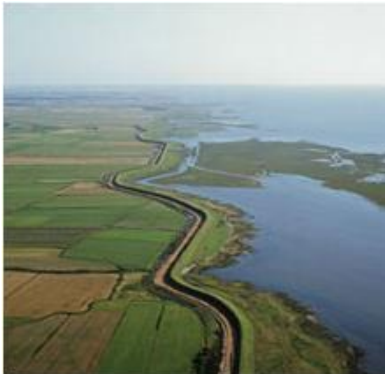
Figure 17.57 The dike in the Danish Wadden Sea, note that the dike is protected by a marshy foreland.
