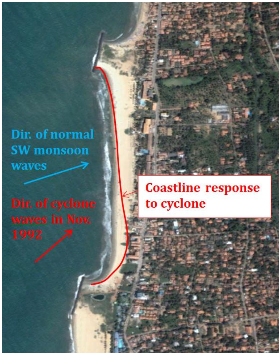
Figure 17.33 Segmented breakwater scheme in Negombo, Sri Lanka including coastline response to cyclone in November 1992.
