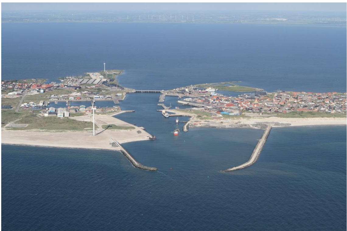
Figure 15.2 Example of a combined tidal inlet and harbour mouth. Hvide Sande, Denmark.
