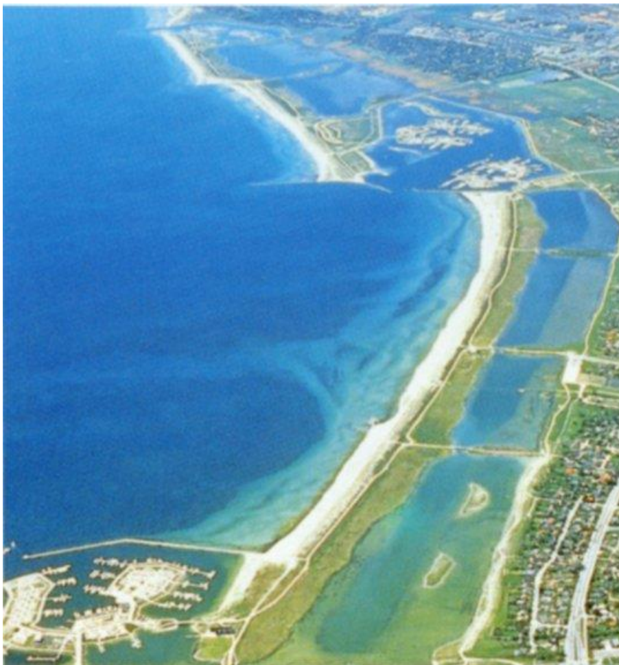
Figure 17.54 An example of a beach park constructed on top of shallow barrier islands by moving the beaches out to deeper and more exposed water combined with a deepening of the lagoon, the construction of marinas, etc., Køge Bay Beach Park, Denmark.
