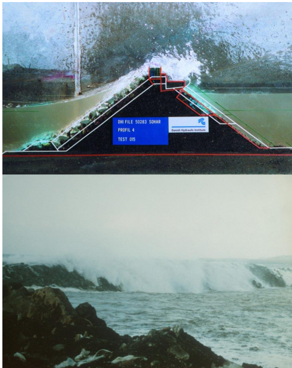
Figure 5.18 Wave-overtopping of breakwater in a flume test (upper) and in nature (lower).
