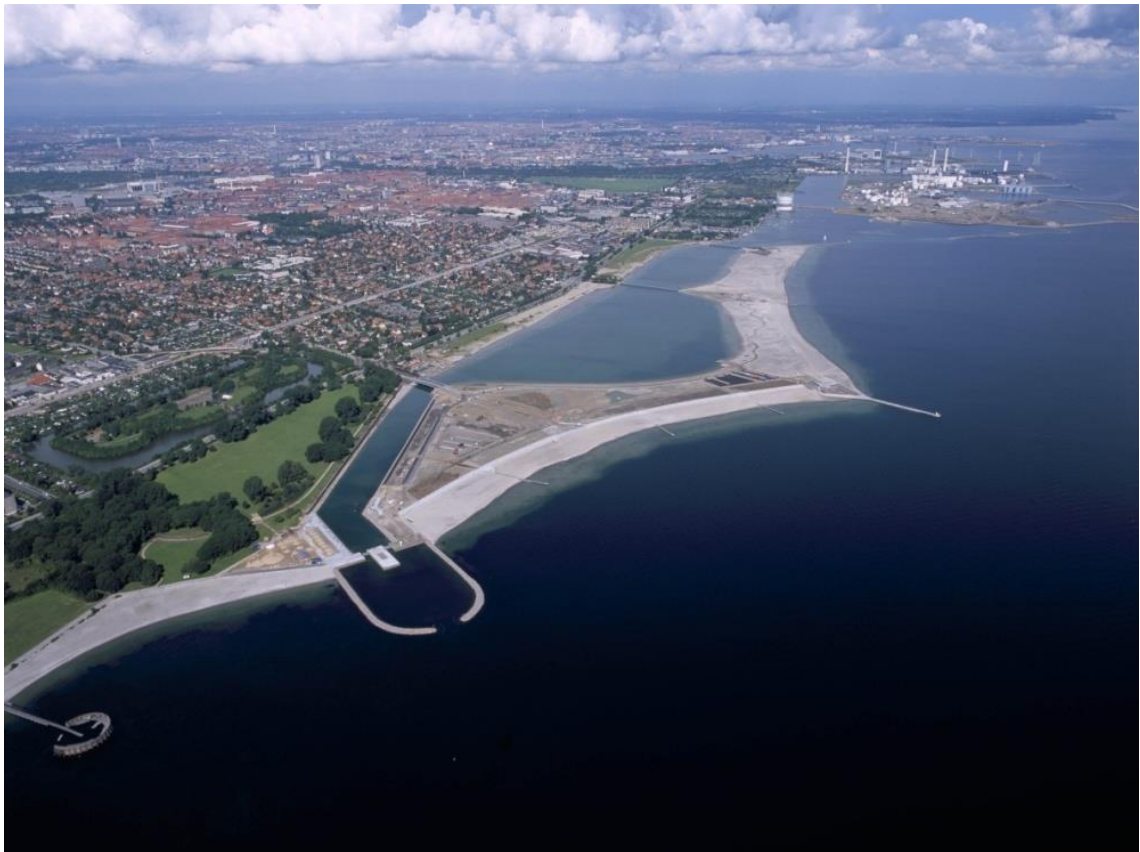
Figure 18.19 Aerial photo of Amager Beach Park (2005), which consists of the following main elements: Island with terminal structures north and south and a separating headland between northern and southern beaches and a lagoon. Designed by DHI, Hasløv and Kjærsgaard and NIRAS.
