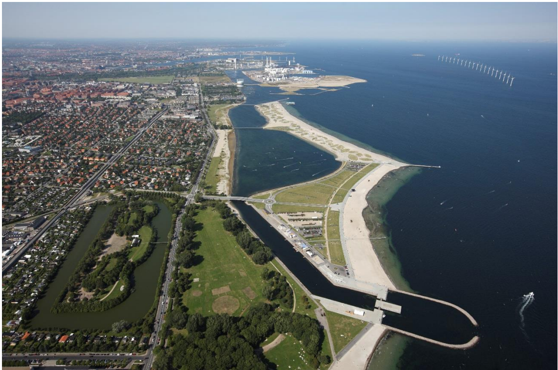
Figure 17.55 At Amager Beach Park, the existing beach was moved seaward on a shallow profile out to an exposed location and an artificial lagoon was excavated. The new beach is divided in two sections each facing one of the two dominant wave directions at the site.
