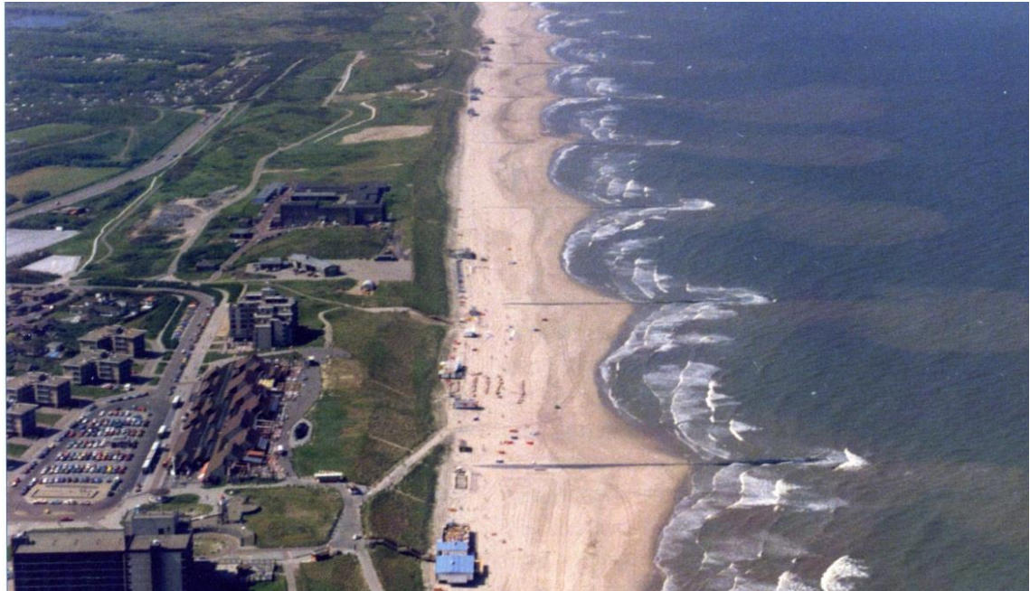
Figure 5.41 Groyne field at Delfland, Holland. The groynes generate rip jets, which transport sand away from the littoral zone. From Terra et Aqua , Number 107, June 2007.
