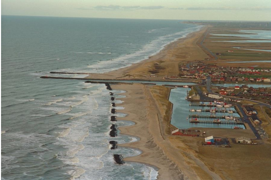
Figure 21.42 A complex shoreline situation around a stabilised tidal inlet with updrift shoreline accretion and a large number coastal breakwaters to stabilise the downdrift coast.
