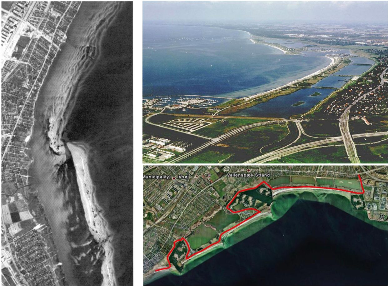
Figure 16.3 Køge Bay Beach Park south of Copenhagen, inaugurated in 1980. Left: Natural conditions. Right Upper: Aerial photo. Right Lower: Satellite image with the alignment of the dike shown as a red line.
