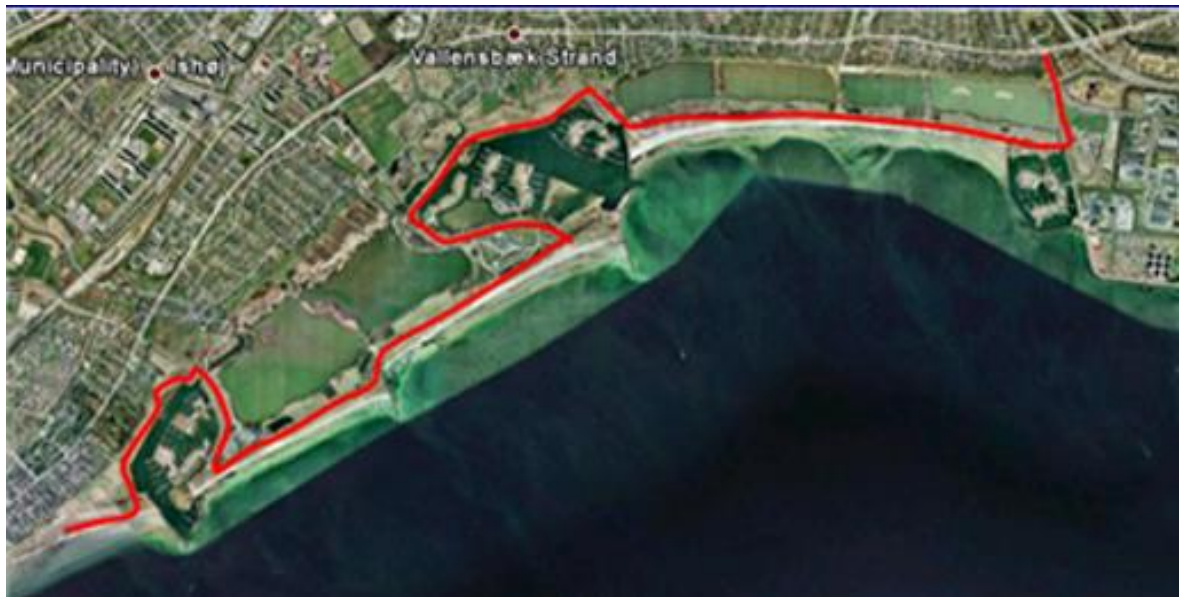
Figure 18.7 Køge Bay Beach Park south of Copenhagen, Denmark. A dike, marked with a red line, is integrated in the dunes and runs behind the marinas thereby protecting the entire hinterland against flooding.
