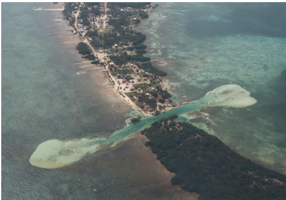
Figure 5.37 Ebb and flood shoals at tidal channel, Cay Calker, Belize. This area is mainly exposed to the tidal currents, whereas the wave climate is very mild.
