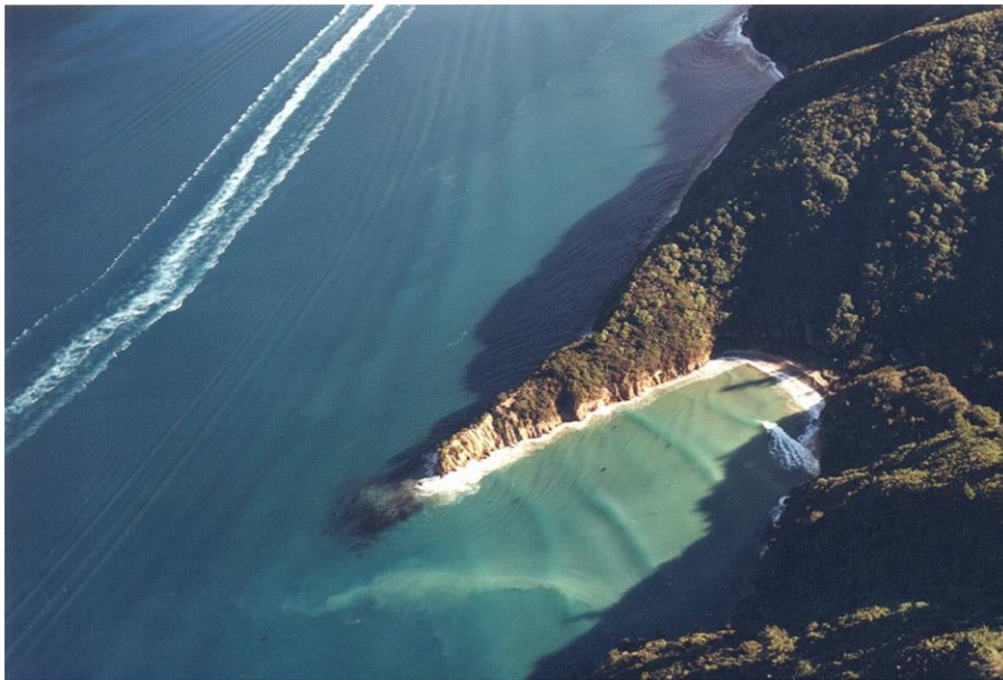
Figure 11.14 Wake waves from a fast ferry in Tory Channel, Queen Charlotte Sound, New Zealand. Note the violent breaking, turbid water and rip currents. (Copyright: Marlborough District Council, photographer: Graeme Matthews).
